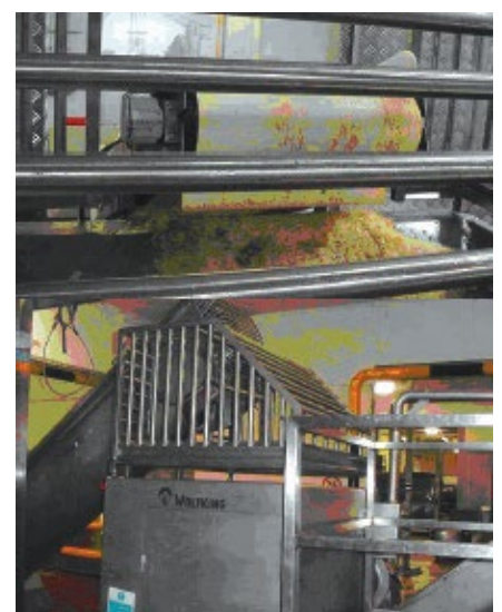
Conveyor and auger fed machines. A fixed or interlocked guard over the top of the hopper/and conveyor can be provided. As shown above
