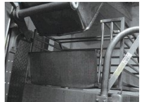
Grinder hopper fenced to accommodate bin lift with extension to reach distance under the bin
