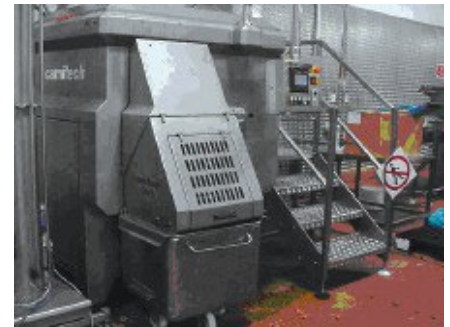
Above. An outfeed hood and interlock bin system. On larger machines for example 11 or 16" diameter worms over-run of the worm can be a problem. A Time-delay device should be fitted in addition to the interlock in such situations.
