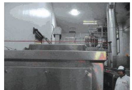
Note red pull cord, which does not prevent access
