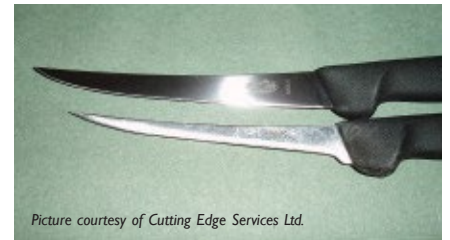
Figure 2: a knife worn to the point where it would be unsafe to use
