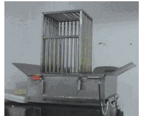
Above an interlocked extended reach guard for hand feeding
